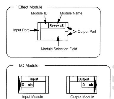
The module can be selected by clicking the module selection field, ID display field, or name field. When selected, the module selection is displayed in black, with its border (frame) emphasized.
