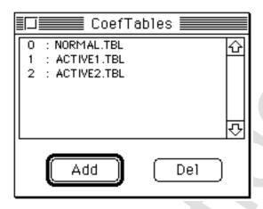
The ADD button is used for registering an additional coefficient table file. The DEL button is used for deleting the coefficient table file in a selection mode. Once a file is deleted, the subsequent coefficient table files will have their numbers shift. Therefore, it is necessary to reassign the coefficient table numbers specified of the modules.
