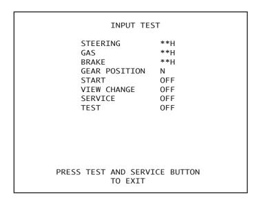
FIG. 9. 3 a INPUT TEST screen
