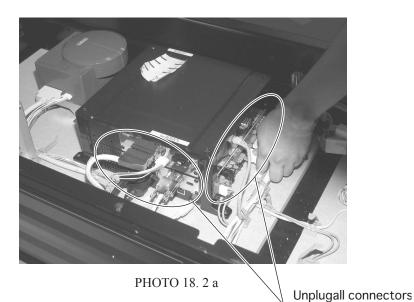
Unplug the AVIP Cable connected to the Chihiro Board.
