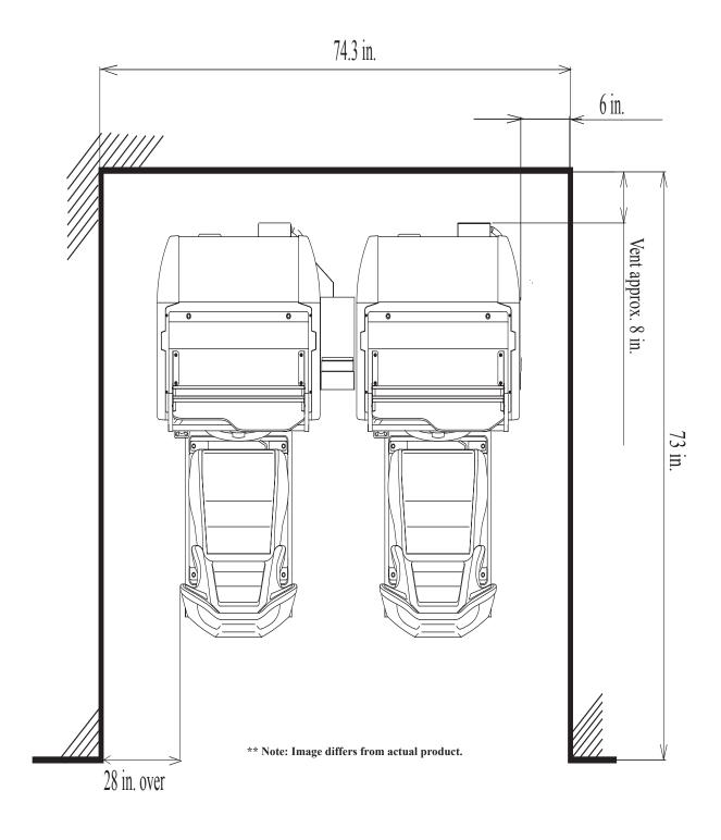
FIG. 6. 2 e Provide ventilation space for the ventilation opening. Allow more than 28 in. of space for customer traffic.
