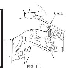
The coin selector should be cleaned once every 3 months. When cleaning, follow the procedure below:
