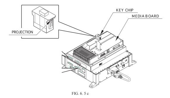
Return the ASSY MAIN BD (now installed with the GD-ROM drive) into the PTV cabinet. Following the above-described actions in a reverse order, fix the base, connect the connectors, and clamp the wires/cables.
