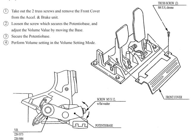
Check Volume values in the Test Mode. Since work is performed inside the energized cabinet, be very careful so as not to touch undesignated portions. Touching places not specified can cause an electric shock or short circuit.
