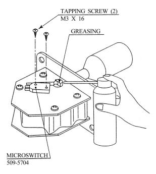
After replacing the Switch, check to see if the switch is inputted as per Shift Lever operation in the Test Mode.
