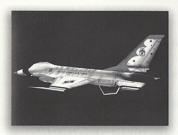
Although only a single-engine aircraft, the engine of the F-16 has strong thrust. The body has a novel construction with the wings blending into the sides. The rudders are now controlled through a computer in a system referred to as "Fly by Wire." With these improvements, the F-16 in certain respects demonstrates performance surpassing the F-15.
