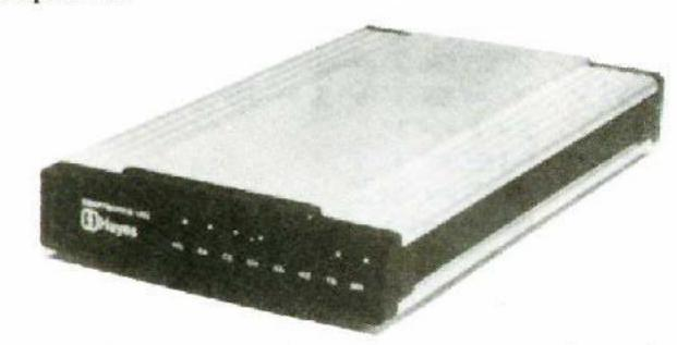
A direct line modem with all the mod cons. (note the facia L.E.D.s to tell the operator what is happening.
