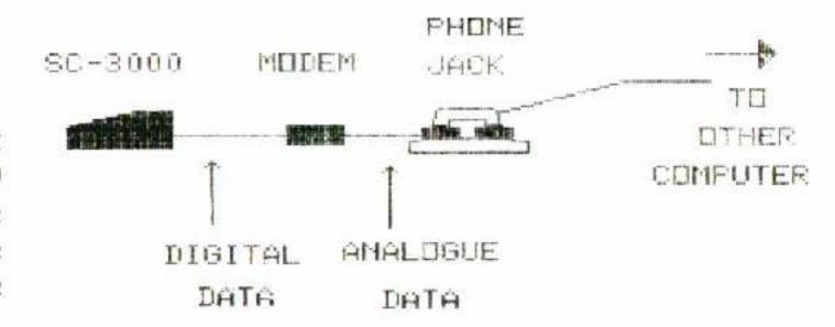
There are two types of modems available, one being a "DIRECT LINE" and the other being an "ACOUSTIC TYPE".
