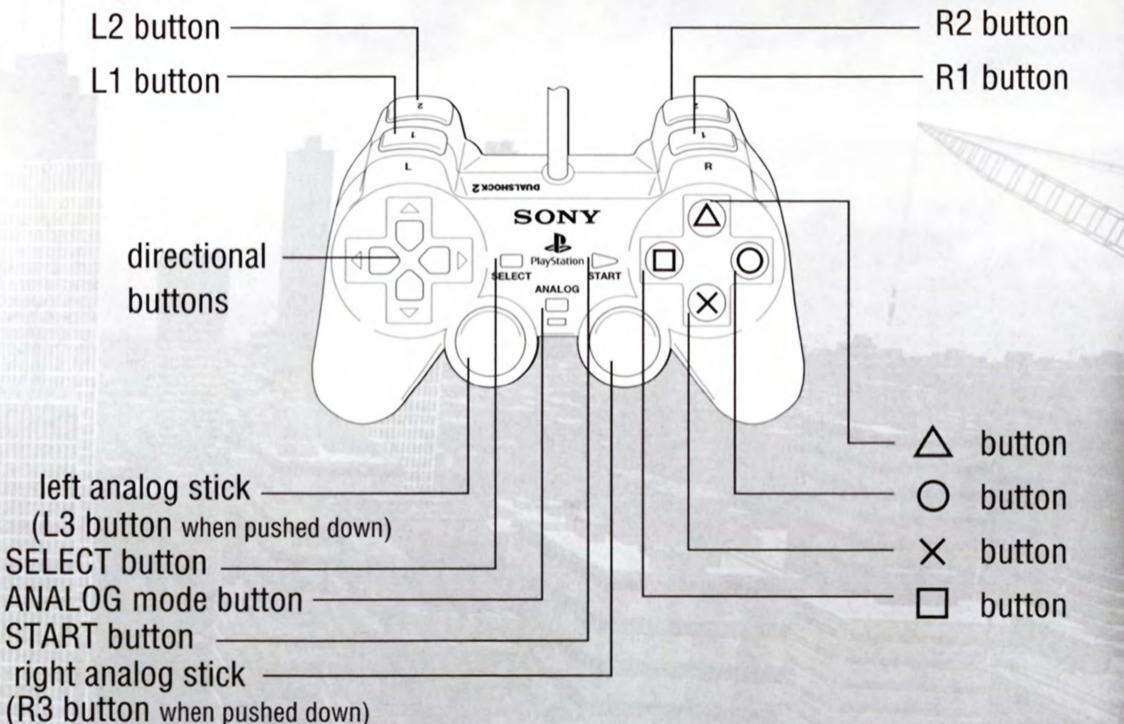
Controls are all set to ANALOG mode (mode indicator: ON) and cannot be switched to digital mode by using the ANALOG mode button.
